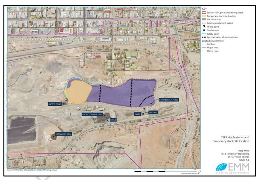
Figure 4 – Temporary tailings Stockpile
