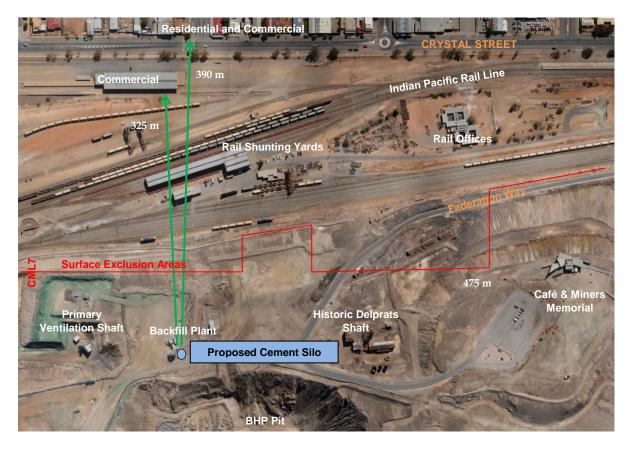
The 300 tonne capacity cement silo would be of steel construction, fabricated off-site and placed in position on-site using a crane. It would be 18 m high and 4.6 m wide. The area would be levelled to provide a base for the footings and concrete slab using an excavator and loader. Construction would
